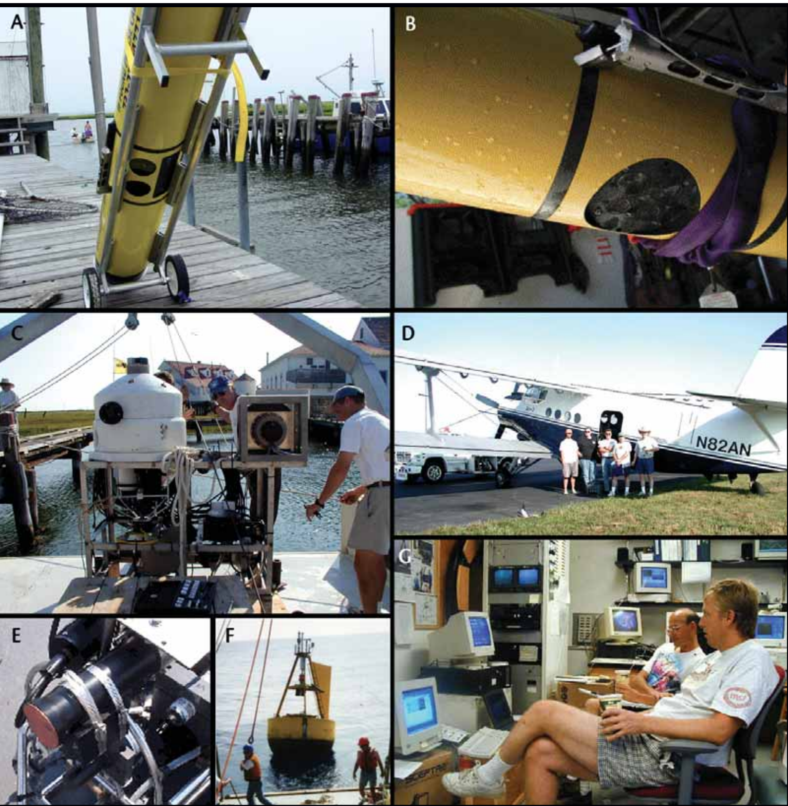
Figure 3. Some examples of now-robust off-the-shelf optical technology during the HyCODE effort that are currently available to oceanographers. (A) A Webb glider ( http://www.webbresearch.com/slocum.htm ) outfitted with an attenuation meter and two backscattering sensors embedded in the belly of the autonomous vehicle. (B) Another Webb glider outfitted with a 2-wavelength backscatter sensor and a fluorometer. (C) A robotic-profiling optical mooring outfitted with absorption-attenuation meters (Wetlabs, Inc.), bioluminescence bathyphotometers, forward-scattering sensors (Sequoia Instruments), and backscatter sensors (HOBI labs and Wetlabs, Inc.). (D) A biplane, one of the world's slowest, outfitted with a hyperspectral, remote-sensing reflectance sensor. The slow speed is ideal for allowing detailed calibration studies. (E) A radiometer (Satlantic) outfitted with a copper shutter. The copper shutters have been demonstrated to be highly effective at minimizing biofouling problems. (F) An optical mooring being deployed by the Ocean Physics Laboratory. (G) Living the dream in the COOL room (Glenn and Schofield, 2003) where scientists can sit and drink coffee while all the data are delivered in near real-time. This capability allows for adaptive sampling (Schofield et al., 2003).
