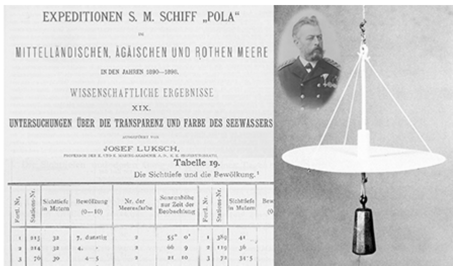
Fig. 2. Josef Luksch (1836–1901) was one of the first oceanographers who frequently used the Secchi disk (on the right) during the Pola expedition in the Mediterranean and Red Sea. Credit: Luksch [1901]
