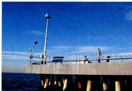
Figure 1. Retractable tower with SeaPRISM and HyperSAS instruments on the LISCO platform.
